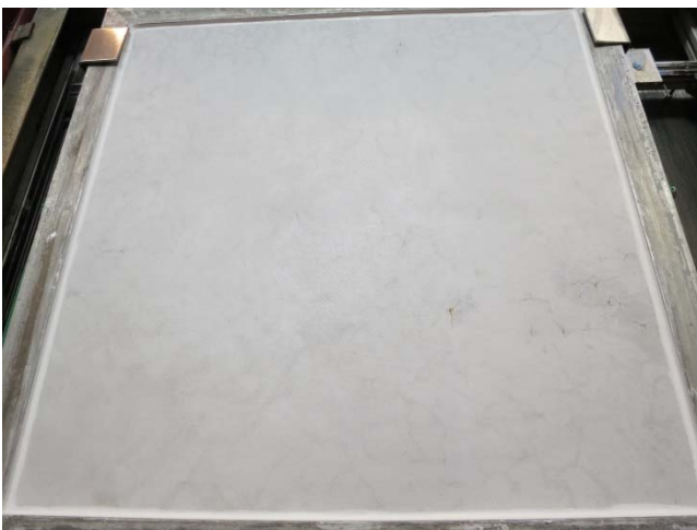
Picture 3: One of the specimens after the initial driving rain test
