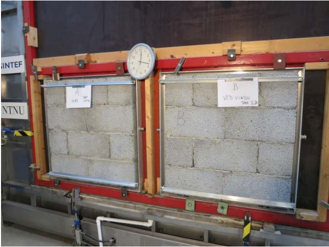
Picture 1: Specimens assembled in the driving rain test chamber before the test was started (unexposed side of the specimens)
