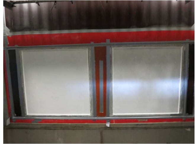
Picture 2: Specimens assembled in the driving rain test chamber before the test was started (exposed side of the specimens)
